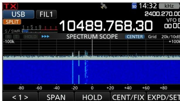
seem possible to “gang” the transmit frequency on 2400 MHz to the receive frequency on 10.489 GHz to allow easy tuning and netting. The absence of any receive capability during transmit made QO-100 operation more difficult.
