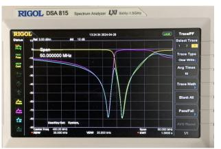
Duplexer factory tuned for 462 & 467 MHz 10dB/div & 5MHz/div
