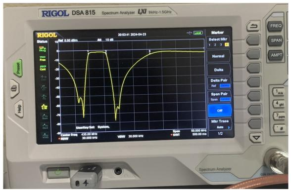
Duplexer tuned as Ch 57 (420-426MHz) ATV Band-Pass Filter 10 dB/div & 5 MHz/div
