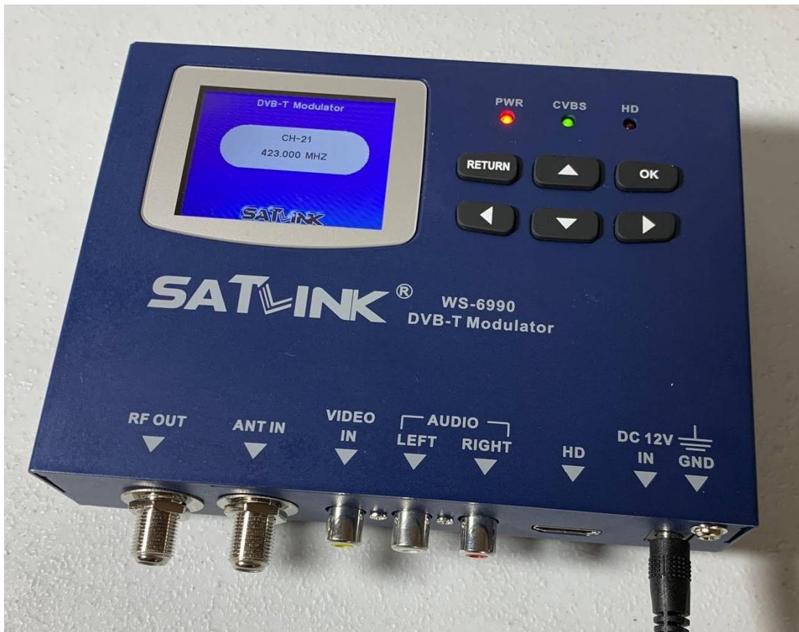
Fig. 1 SatLink model WS-6990 DVB-T Modulator
