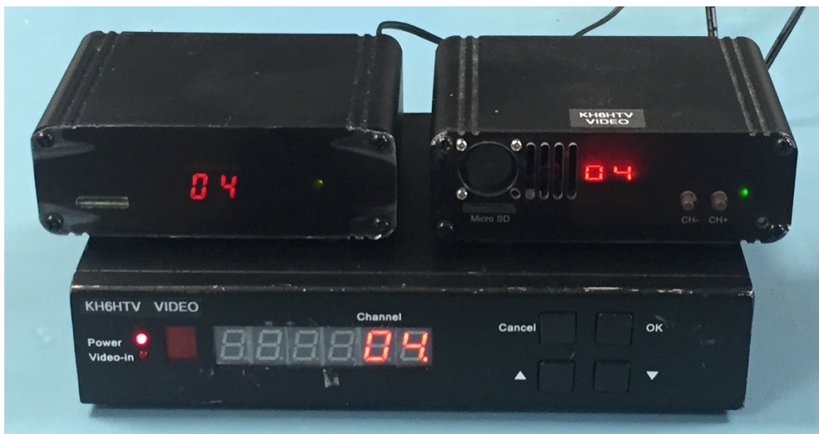
Fig. 1 --- Hi-Des, DVB-T, Modulators. Front View. Bottom is HV-100EH. Top Left is HV-310E. Top Right is HV-320E
