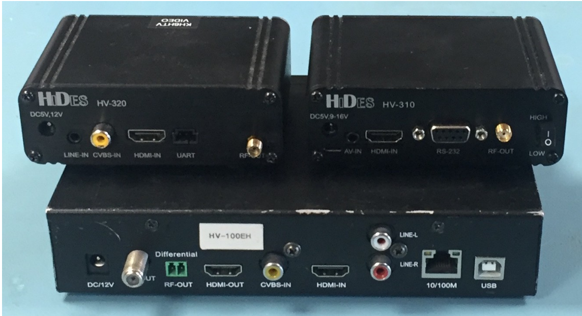
Fig. 2 --- Hi-Des, DVB-T, Modulators. Rear View. Bottom is HV-100EH. Top Right is HV-310E. Top Left is HV-320E
