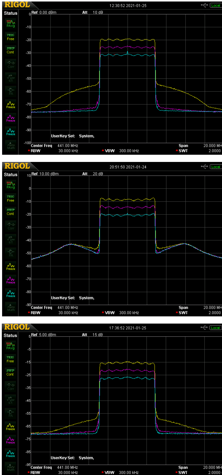
Fig. 3 --- Comparison of modulator spectrums for a 70cm DVB-T signal with 6 MHz bandwidth. Top = HV-100EH, Middle = HV-310E & Bottom = HV-320E. Spectrum analyzer settings per ITU specs. Center frequency = 441 MHz, 10dB/div & 2 MHz/div. Yellow = Max. RF output Magenta = -6dB & Cyan = -12dB
