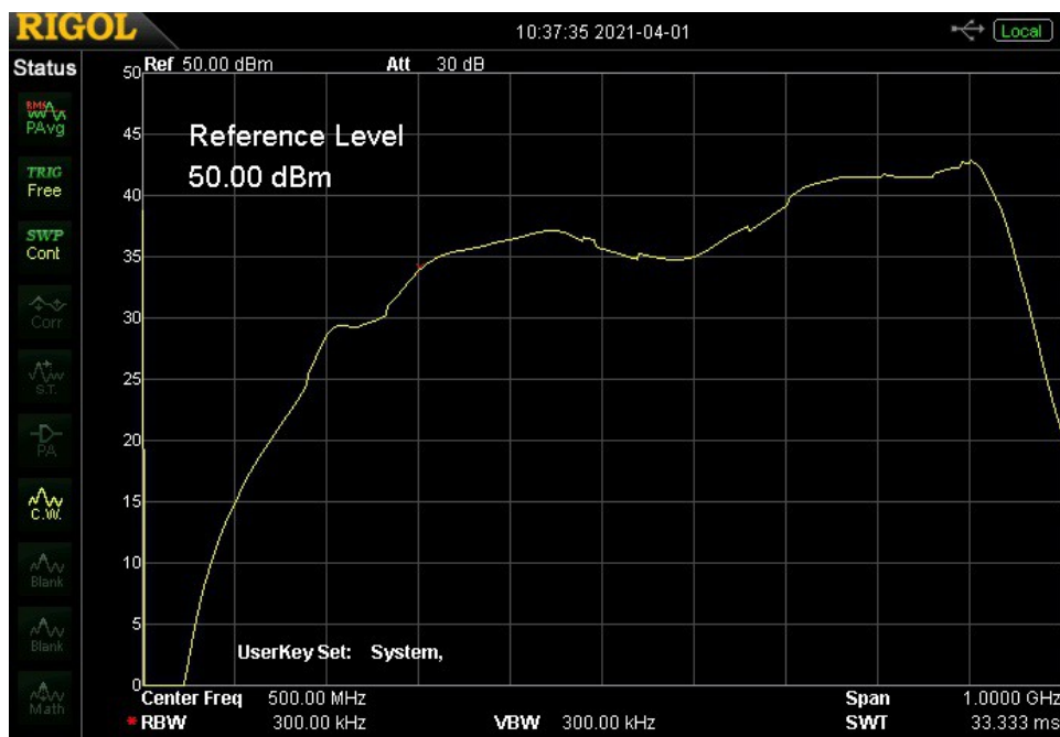
Max. Power Output with Pin = 0dBm. Sweep from to 1 GHz. 5dB/div & 100MHz/div
