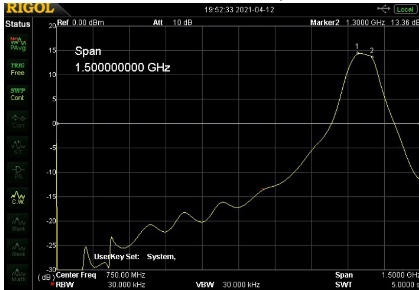
S21 vs. Frequency -- sweep from 0 to 1.5GHz, 5 dB/div & 150 MHz/div. markers 1 & 2 show 23 cm band edges
