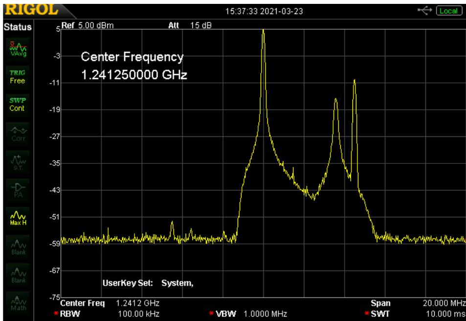
Fig. 9 Up-Conversion of VUSB-TV signal from 70cm band to 23cm band. Top photo is IF input at 421.25MHz. Bottom photo is RF output at 1241.25 MHz. 20 MHz span, 8 dB/div & 2 MHz/div. The video test signal was NTSC color bars. The up-conversion gain is +13dB.
