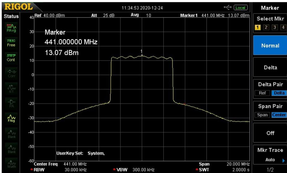
This photo now shows doing the measurement on the 3 Watt output from the 70-7B amplifier. This was the same signal used to evaluate the Bird and Micro-Match power meters. Applying the +22dB correction factor to the above measured +13dBm, we can estimate the rf power to be about +35dBm ( 3.2 Watts). This technique is not as accurate as using a thermistor rf power meter, but will give close correlation.
