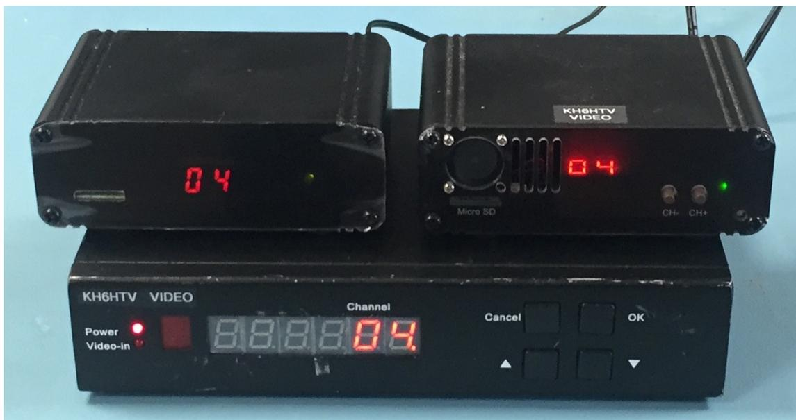
Fig. 1 --- Hi-Des, DVB-T, Modulators. Front View.
