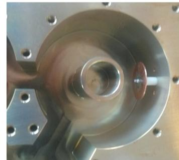
Dan pre-tuned the filter by setting the tuning screws to his design dimensions. He then tested the BPF on a vector network analyzer. His predictions were extremely close. The initial passband was only about 4 MHz too high. The plot below of S21 and S11 shows the results after he then fine tuned the filter. The traces in blue are the theoretical predicted responses while the red traces are the actual measured performance after fine tuning.
