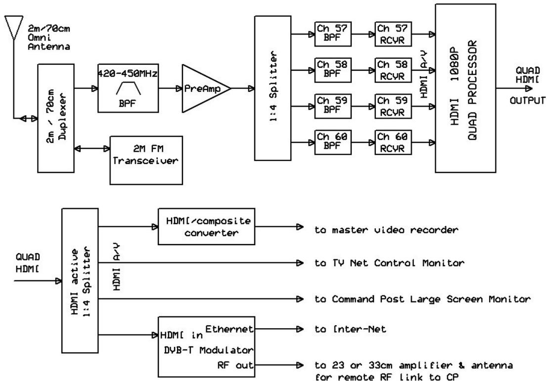
Fig. 4 Block Diagram of BCARES, Quad DVB-T Receiver
