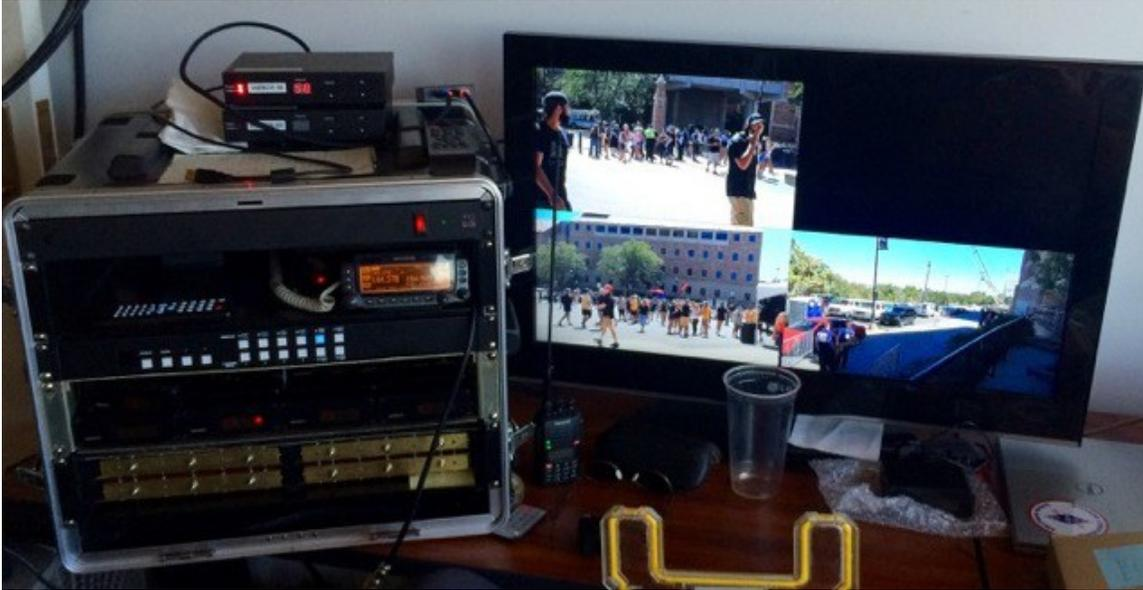
Fig. 2 The new BCARES Quad DVB-T Receiver and live, hi-defination images at a CU football game received on channels 57, 58 & 60. Note: ch. 59 is also possible.
