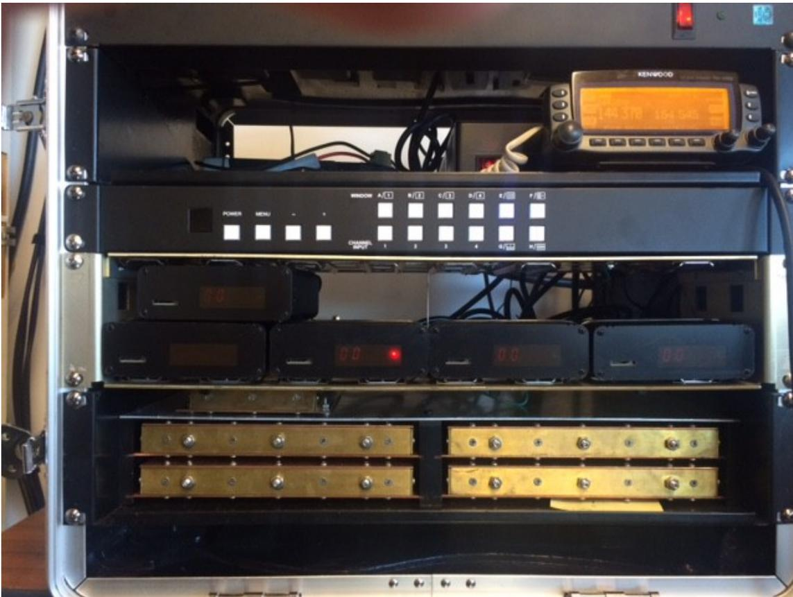
Fig. 3 Close up of the front of the new Quad DVB-T Receiver. Key items seen top to bottom are the 2m FM transceiver, the HDMI quad processor, 4 Hi-Des DVB-T receivers, and 4 Spectrum International band-pass, channel filters.
