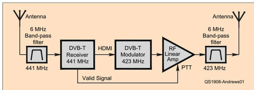
Figure 1 — Block diagram of a DVB-T repeater.
