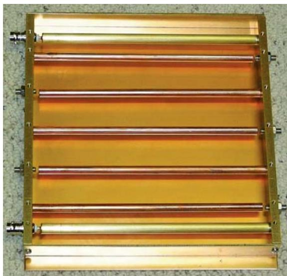
**Figure 2** — An interdigital band-pass filter for 70 centimeters. The top cover is removed to show construction. [Jim Andrews, KH6HTV, photo]
