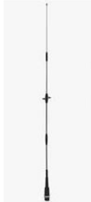
The Comet specs. for the antenna were: VSWR < 1.5:1 144-148 & 440-450 MHz, VSWR < 2:1 140-160 & 435-465MHz, Gain = 3.8dBi (2m) & 6.2dBi (70cm), 150 watts max., length = 40", NMO or PL-259 connectors available. The optional spring, model CA-SPR was ordered and installed in the antennas.
