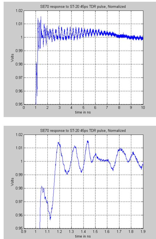
**Fig. 3** SE-70's blow-by response to 45 ps TDR pulse. Settling time to 0 V topline expanded. 1%/div & 10 ns time window (top) & 1 ns (bottom). Ringing is generator artifact.
