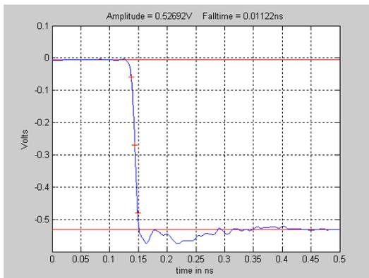
**Fig. 4** NPL calibration data for PSPL's gold standard, model 4015C pulse generator.  $T_{fall} = 11.2$  ps.
