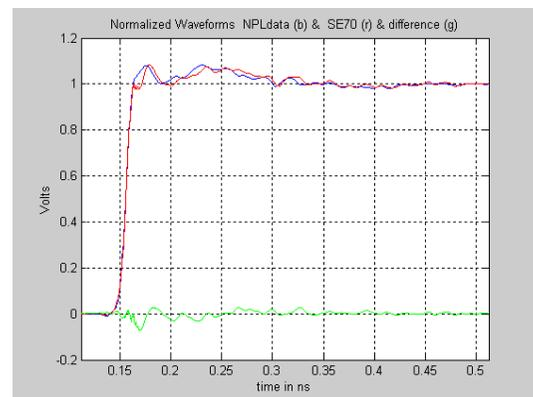
**Fig. 10** 4015C waveforms. Comparison of normalized NPL data (blue) and deconvolved SE-70 measurement (red). Difference (green).
