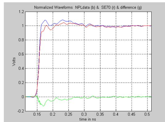
**Fig. 6** Comparison of normalized NPL data (blue) and the 4015C waveform measured by the SE-70 sampler (red). Difference (green).
