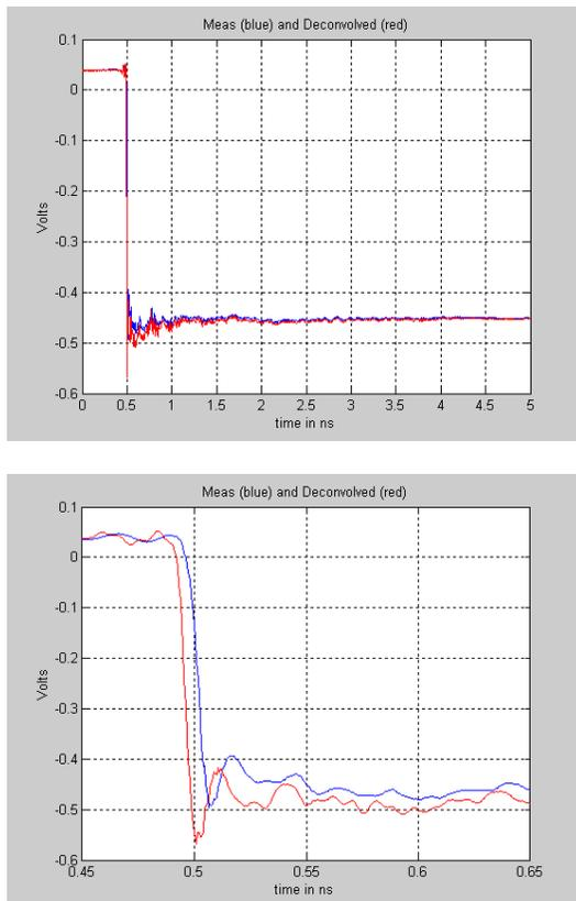
**Fig. 12** Deconvolution (red) of PSPL 4016 pulser. Measured waveform (blue), Deconvolved waveform (red), 5 ns (top), and 200 ps (bottom) time windows.
