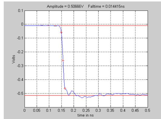
**Fig. 5** SE-70 measurement of above NPL calibrated 4015C.  $T_{fall} = 14.2$  ps.
