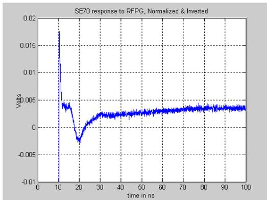
**Fig. 2** SE-70 blow-by response to RFPG, expanded vertical = 0.5% /div, 100 ns time window.
