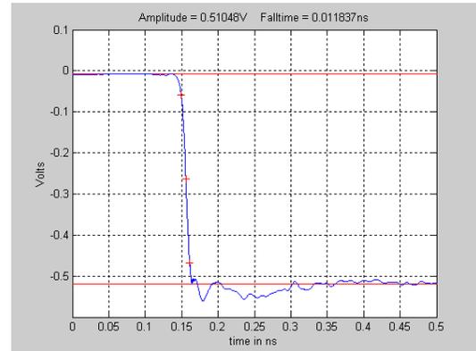
**Fig. 9** Deconvolved 4015 waveform.  $T_{fall} = 11.8$  ps.
