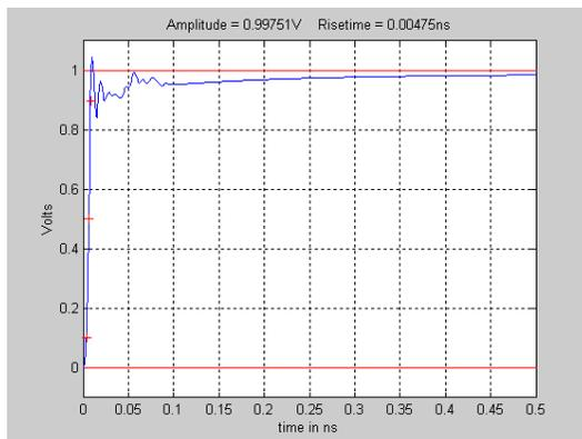
**Fig. 8** Gold Std. SE-70 step response including PTB calibration data and modeled Blow-by effects. 500 ps time window.  $T_{rise} = 4.75$  ps.
