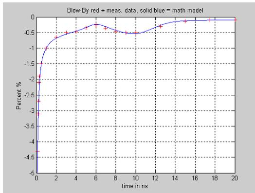
**Fig. 7** Blow-By correction math model for Gold Std. SE-70 sampler. Blue trace is math model. Red crosses are measured blow-by data. 20 ns time window.
