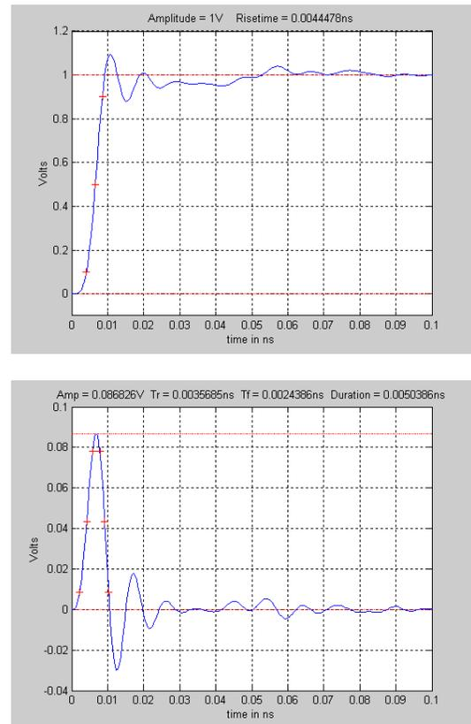
**Fig. 1** PTB step response (top) and impulse response (bottom) calibration data for PSPL's Gold Std. SE-70 sampling head. Step  $T_{rise} = 4.4$  ps & Impulse  $T_d = 5.0$  ps.
