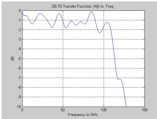
**Fig. 11** Frequency response of Gold Std. SE-70 sampling head.
