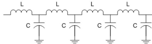
Fig. 11 Transmission Line Model
