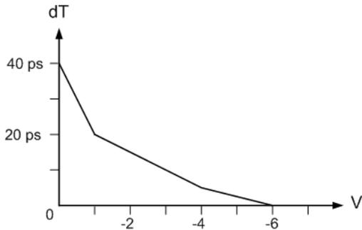
Fig. 13 Typical NLTL time delay shift vs. voltage
