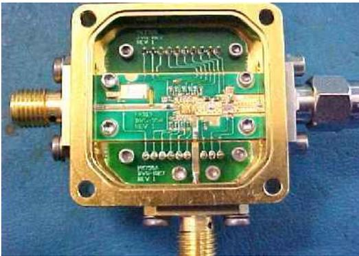
Fig. 14 PSPL custom designed Ultra-Broadband, 25 GBit/s, 2 V, 20 ps rise/falltime, Amplifier, MMIC.
