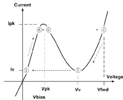
Fig. 9 Tunnel Diode I - V Curve
