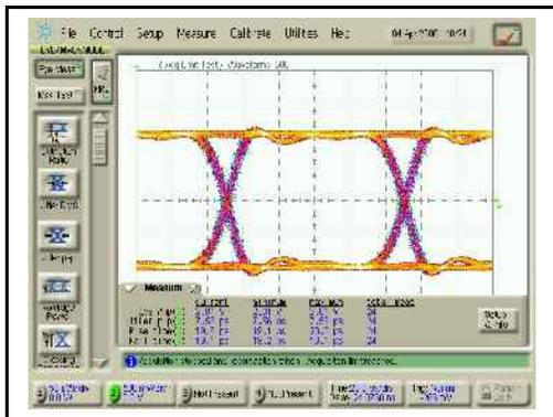
Fig. 3 PSPL, custom MMIC, Programable Pattern Amplifier 10 GHz PRBS, NRZ eye diagram 0.5 V/div & 20 ps/div
