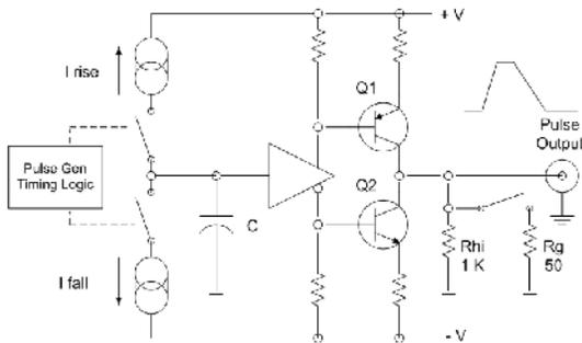
Fig. 5 Ramp generator & linear amplifier to generate adjustable rise/falltime pulses.
