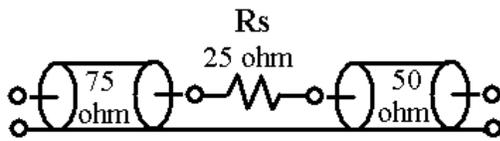
Fig. 5 One-way 25  $\Omega$  series matching resistor
