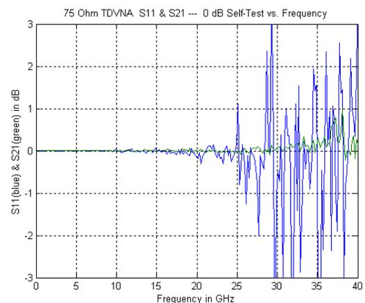
**Fig. 15** 75 $\Omega$  TDVNA 0 dB self-test of repeatability and maximum frequency;  $S_{21}$  (green) and  $S_{11}$  (blue)
