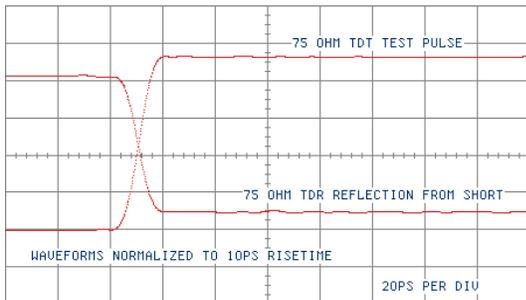
**Fig. 13** 10 ps normalized TDT and TDR test pulses, 20 ps/div
