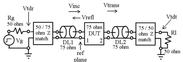
**Fig. 4** 75 Ω TDT and S<sub>21</sub> TDVNA, using Z matching networks and 50 Ω test equipment
