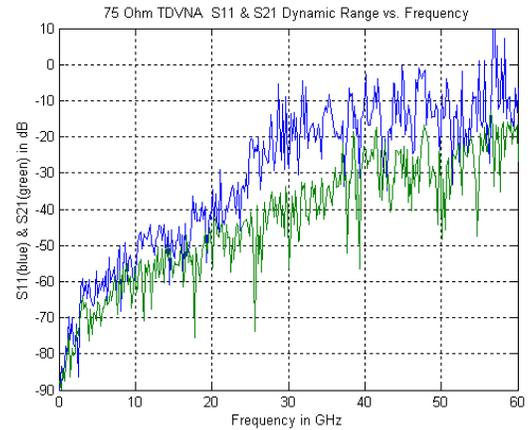
**Fig. 14** 75 $\Omega$  TDVNA system self-test for dynamic range;  $S_{21}$  (green) and  $S_{11}$  (blue)
