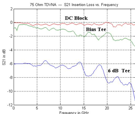
**Fig. 16**  $S_{21}$  of 75 $\Omega$  broadband coaxial components; DC Block (red), Bias Tee (green), and 6 dB Tee (blue)
