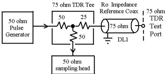
Fig. 9 Special 75  $\Omega$  TDR Tee for use in a 50  $\Omega$  system
