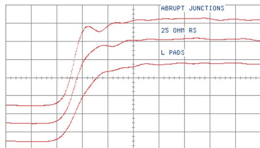
Fig. 11 75  $\Omega$  TDT test pulses with various Z matching networks, 100 mV/div and 20 ps/div
