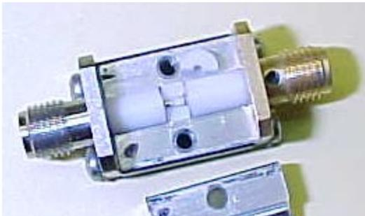
Fig. 7 75  $\Omega$  to 50  $\Omega$  series matching resistor. The 25  $\Omega$  chip resistor is mounted between the center pins of the 75  $\Omega$  and 50  $\Omega$  coax connectors.
