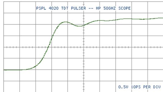
Fig. 10 PSPL 4020 TDR pulser measured on HP 50 GHz oscilloscope, 0.5 V/div and 10 ps/div
