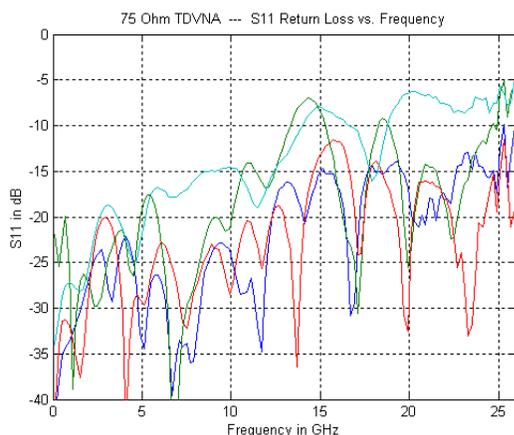
**Fig. 17**  $S_{11}$  of 75 $\Omega$  broadband coaxial components; DC Block (red), Bias Tee (green), 6 dB Tee (blue), and 25  $\Omega$  Series, 75 to 50  $\Omega$  Terminator (cyan).
