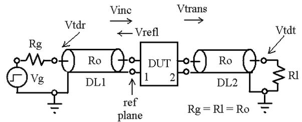
**Fig. 3** Basic TDR, TDT and TDVNA Measurement Set-up
