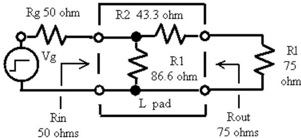
**Fig. 2** Minimum Loss 50 / 75 Ω "L" Matching Pad
