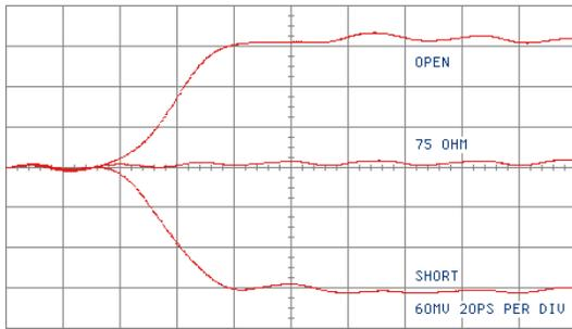
**Fig. 12** 75  $\Omega$  TDR — reflections from open, 75  $\Omega$ , and short; 60 mV/div & 20 ps/div
