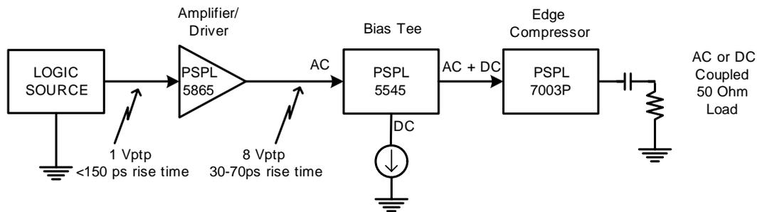
**Figure 11: Using a Model 5865 Amplifier/Driver to Boost Logic Signal Levels**
