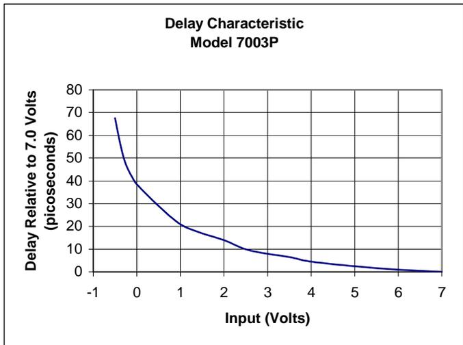
**Figure 3: Delay of 7003P Edge Compressor versus Input Voltage (relative to +7 volts)**
