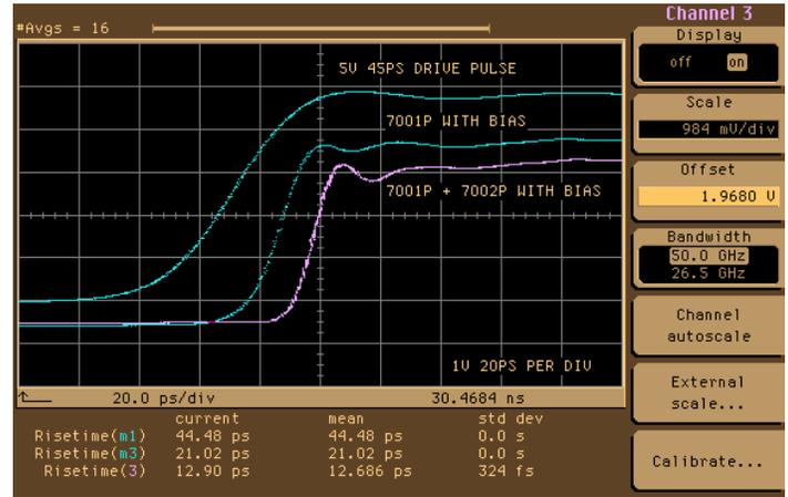
**Figure 6: Pulse Edge Compression with Cascaded PSPL Models 7001P and 7002P**
