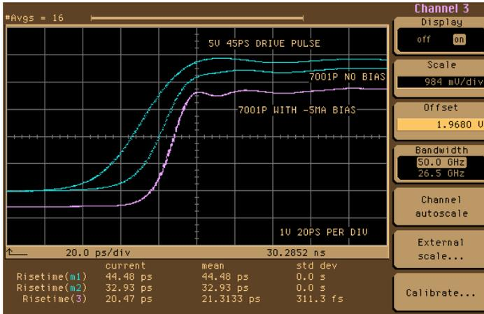
**Figure 5: Edge Compression Using a PSPL Model 7001P**
