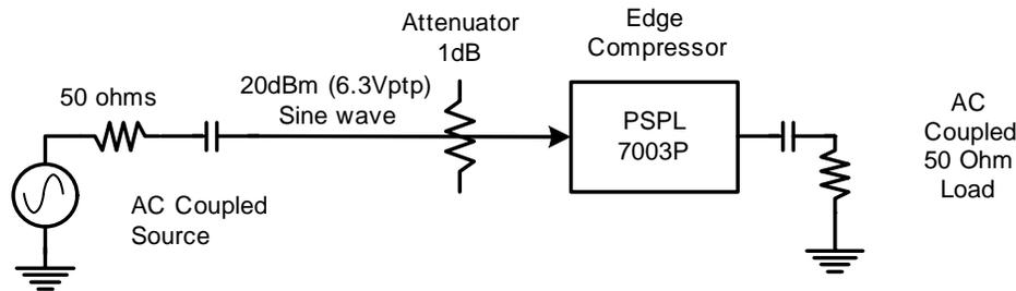
**Figure 9: Sine Wave Drive without Bias Tee**
