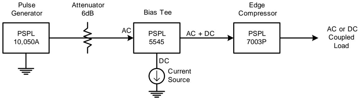
**Figure 7: Pulse Drive with Bias Tee**
