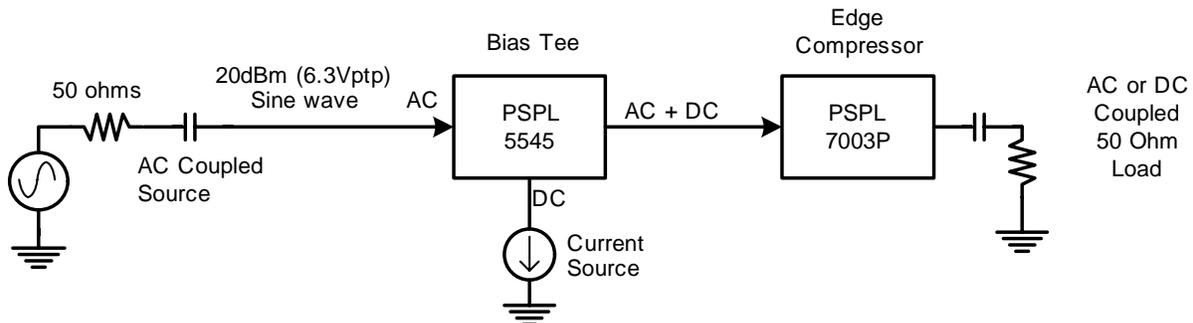
**Figure 8: Sine Wave Drive with Bias Tee**
