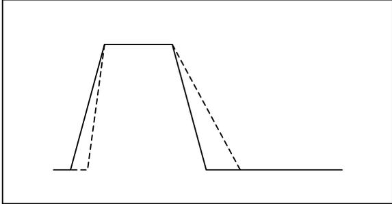
**Figure 4: The Positive Polarity Edge Compressor Reduces the Risetime and Increases the Fall Time.**
