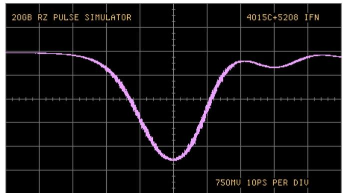
**Figure 11: Simulated 10 Gb/s RZ impulses from PSPL 4050B and 4015C pulse generators**
