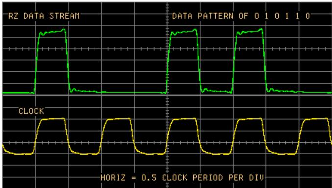
Figure 2: An RZ data stream plus clock
