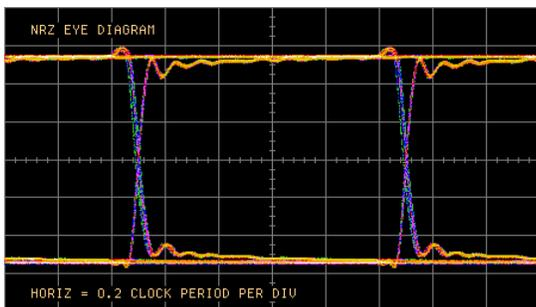
Figure 5: Nearly ideal eye diagram of NRZ data
