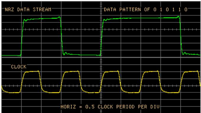
Figure 1: An NRZ data stream plus clock
