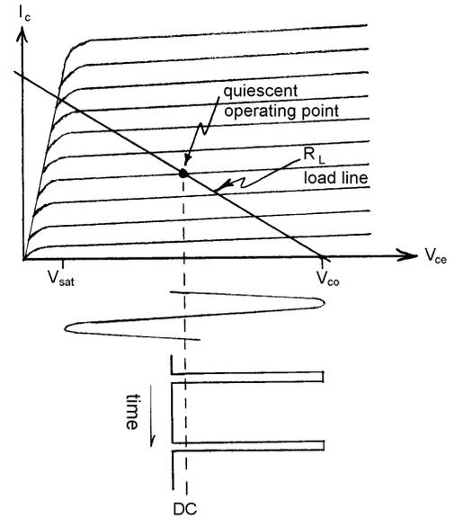
**Figure 15: A Typical class A amplifier load line analysis**
