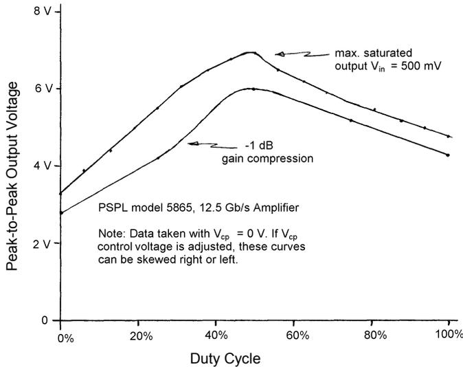
**Figure 14: Amplifier max. output amplitude vs. input signal duty cycle**
