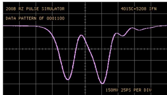
**Figure 13: Simulated 10 and 20 Gb/s RZ pattern sequences of 0 0 0 1 1 0 0, using PSPL impulse generators**
