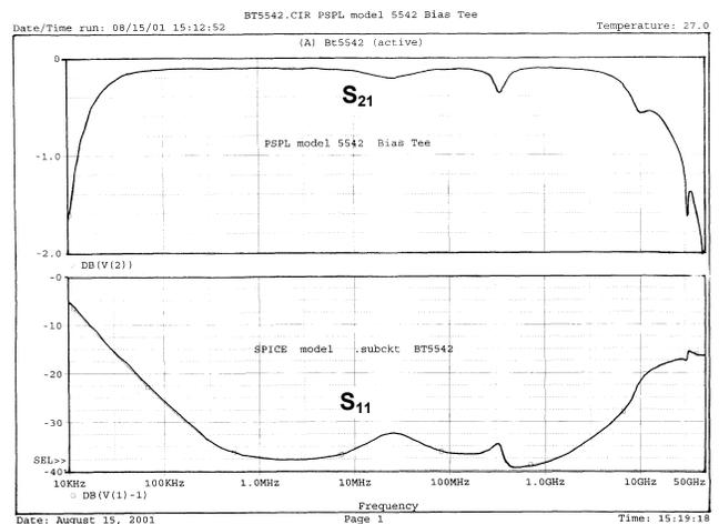
Figure 1: Computed  $S_{21}$  &  $S_{11}$  from .subckt BT5542
