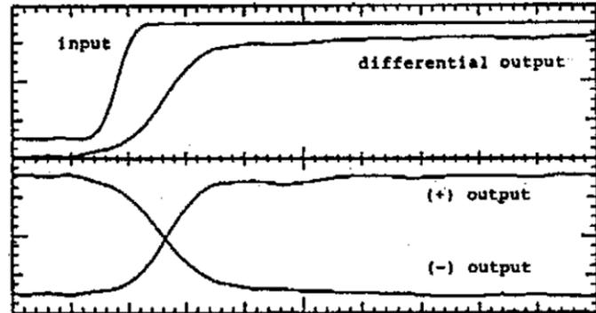
**Figure 4: PSPL Model 5320A BALUN Pulse Response**
