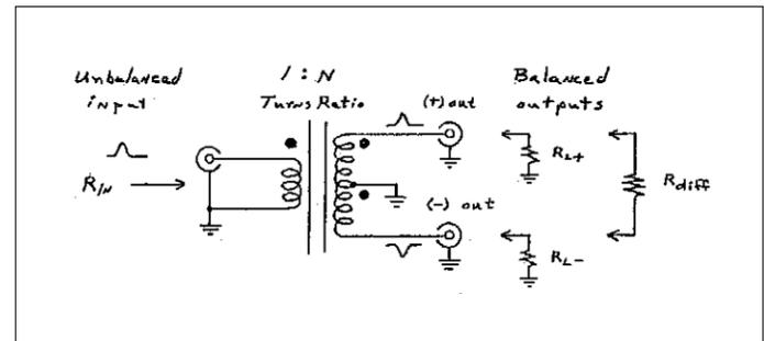
**Figure 2: BALUN Transformer with Center-Tapped Output**
