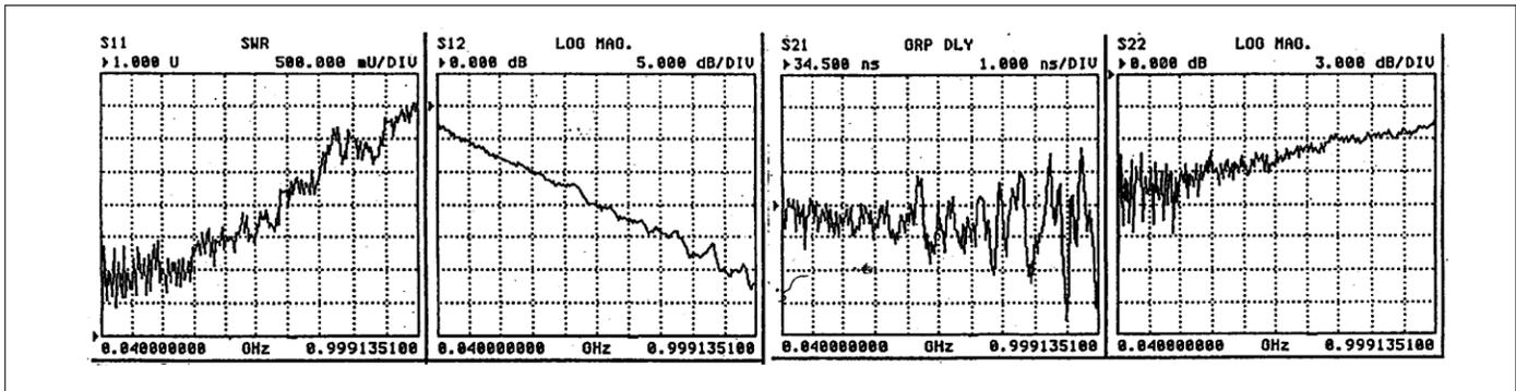
**Figure 11: Differential Measurements of a Shielded #24 Twisted Wire Pair Cable**
