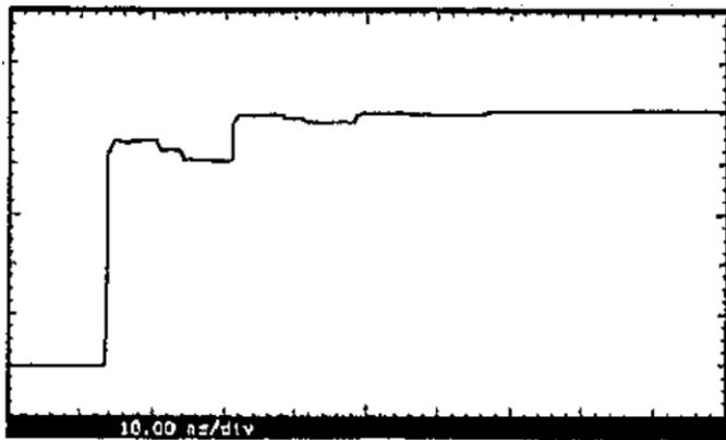
**Figure 5: Pulse Step Response of two 5320A BALUNs Connected Back-to-Back. 10 ns/div.**
