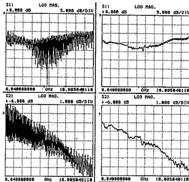
**Figure 6: High Frequency Response of two PSPL 5320A BALUNs Connected Back-to-Back**
