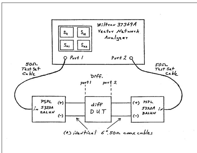
**Figure 8: PSPL/Wiltron, 100 Ohm Differential, 10 GHz Vector Network Analyzer, Test Set**
