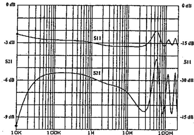
**Figure 7: Low Frequency Response of two 5320A BALUNs Connected Back-to-Back**
