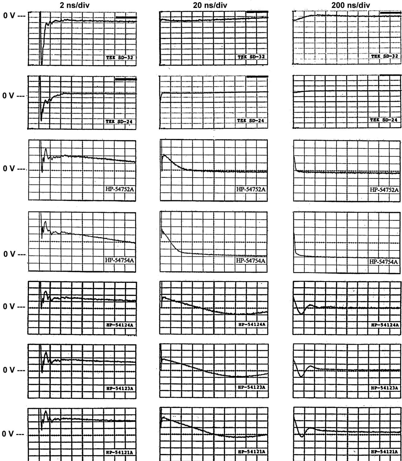
**Figure 3: Nanosecond Domain Settling Time Response of Various HP and TEK Digital Sampling Oscilloscopes**
