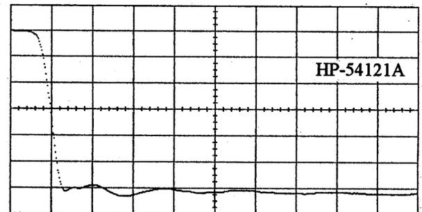
**Figure 2: Measurements of PSPL Model 4015B, -300 mV, 13 ps Step Pulse by Various TEK and HP Digital Sampling Oscilloscopes**
