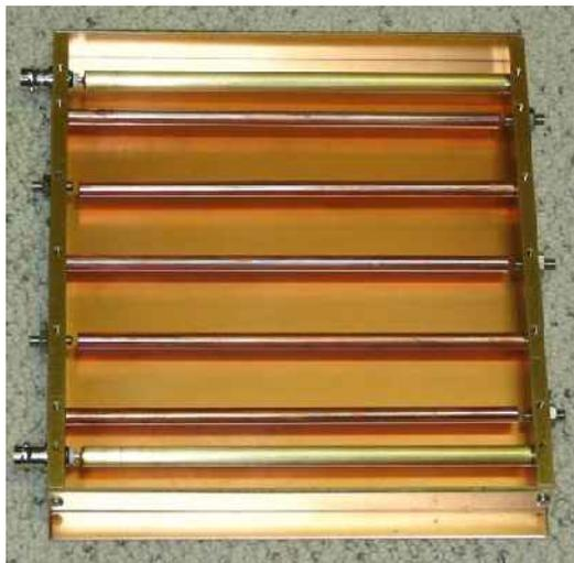
Fig. 2 Typical, 70cm, Inter-Digital Band-Pass Filter. Shown with top cover removed.
