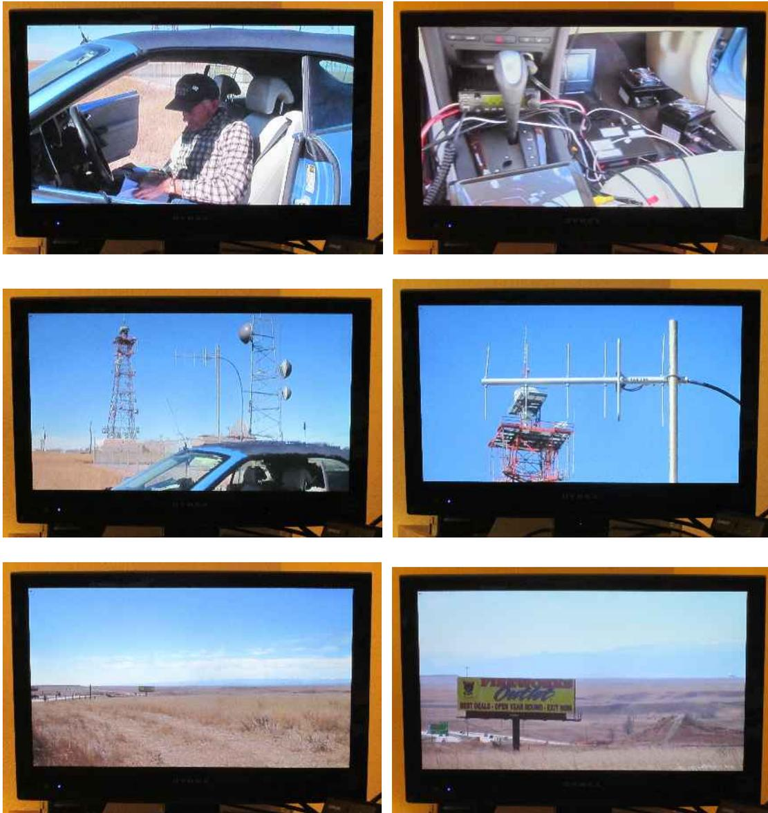
Fig. 6 Various Live high-definition, 1080P images received by N0YE in Boulder, CO from KH6HTV in Cheyenne, WY. A Canon hi-def, 1080P, camcorder was used. Images are of KH6HTV in Saab convertible, the "jumble" of electronics gear on the floor of the car, the AT&T microwave tower and Cheyenne TV towers, close up of 70cm, 6 element transmitting yaggi antenna, wide-angle view to south towards Boulder 77 miles away, with I-25 in left side of photo, and telephoto view to the south.
