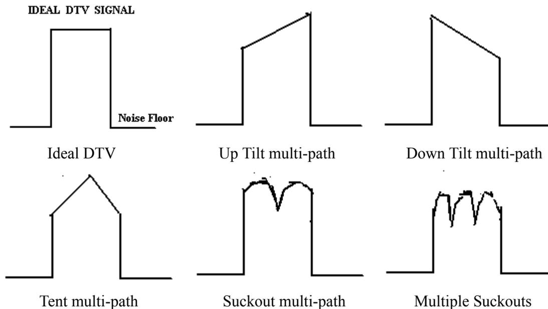
Fig. 6 Examples of various types of multi-path effects on a DTV signal spectrum.
