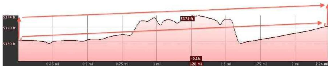
Fig. 5 Example of a bad path that can be corrected with tall antennas.
