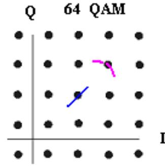
Fig 3. Amplitude & Phase Errors
