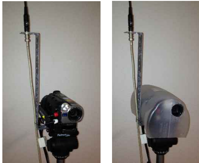
Fig. 1 ARES TV camcorder on a camera tripod with antenna mount [3] --- (left) normal configuration and (right) with protective rain cover.
