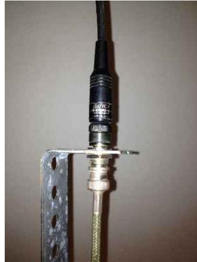
Fig. 4 BNC antenna connector
