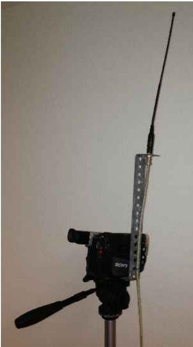
Fig. 1 Antenna Bracket on tripod
