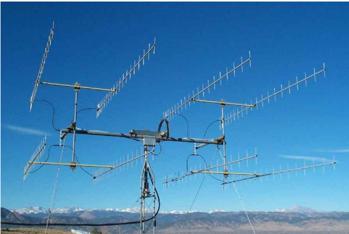
Bill, K0RZ's 70 cm phased array of eight, 22 element yaggi antennas. Gain = 27 dBi (photo courtesy of K0RZ)
