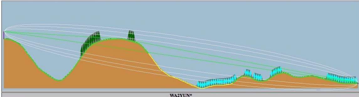
Fig. 5 TV repeater to WA2YUN -- this is an example of an obstructed, short, 1 mile path in which a signal can still be received via diffraction. Pr = -85.9dBm (predicted) & -81dBm (measured) +4.9dB difference
