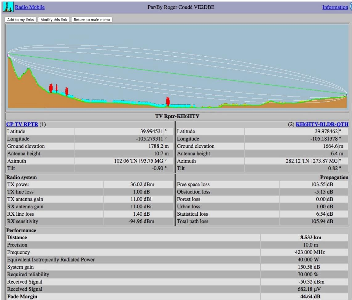
Fig. 2 *Radio Mobile* - Path Profile prediction for TV Repeater to KH6HTV-QTH. Direct line-of-sight, 5.3 mile path between transmitter and receiver. The transmitter is always plotted on the left and the receiver is always plotted on the right side. The green trace is the direct ray. Note: 1st, 2ed & 3ed Fresnel zone ellipsoids (white lines) and intermediate path obstructions are shown.
