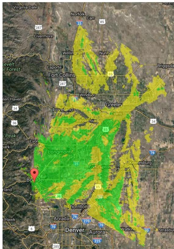
Fig. 1 Boulder, Colorado TV repeater maximum coverage area with an excellent receiving antenna, 11dBi yaggi at 30 ft -- Yellow = >-92dBm, Green = >-82dBm, 100km radius, resolution = 200m/pixel. The red tear-drop indicates the location of the transmitter.
