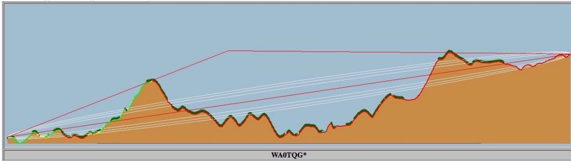
Fig. 8 TV repeater to WA0TQG -- This is an example of an impossible, 6.2 mile path over tall mountains. Transmitter on left at 5,900ft. Receiver on right at 7,400ft. When the direct rays are plotted in red, it indicates the signal strength is below threshold by more than -3dB. Pr = -130dBm (predicted)
