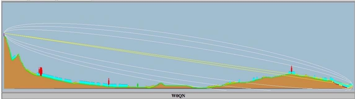
Fig. 7 TV repeater to W0QN -- this is an example of an obstructed, 8.2 mile path in which the received signal is within  $\pm 3$ dB of receiver sensitivity threshold. This is indicated by the direct rays being plotted in yellow. Pr = -89.3dBm (predicted) & -92dBm (measured) -2.7dB difference
