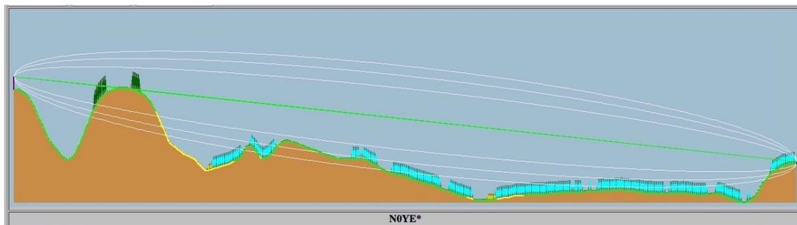
Fig. 4 TV repeater to NOYE --- this is an example of the direct, 2.3 mile path making a grazing pass over an intermediate obstruction. Also note the presence of forested areas on this ridge line (dark green trees). Also noted is urban clutter represented by the small turquoise colored cubes down in the valley and also at the receive site.  $Pr = -70.7\text{dBm}$  (calculated) &  $-70\text{dBm}$  (measured). +0.7dB difference
