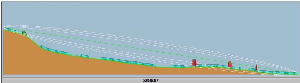
Fig. 6 TV repeater to K0HEH -- this is an example of the direct, 1.6 mile path being obstructed by tall buildings on the Univ. of Colorado campus. They are indicated by the bright red structures. In this case reception was possible due to diffraction in the first Fresnel zone. Pr = -53.7dBm (predicted)
