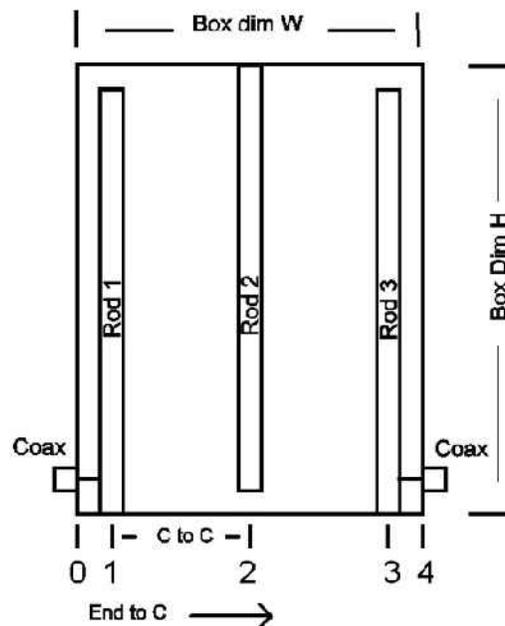
Fig. 8 Basic mechanical design of N6JH ID-BPF with taped input/output on first & last resonator rods.
