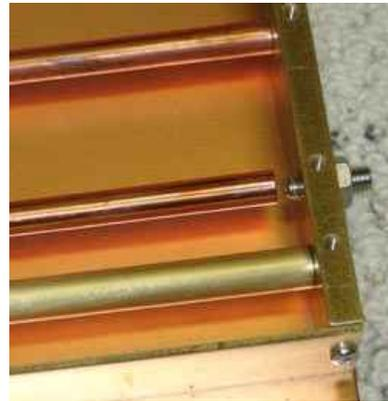
Fig. 5 Close up detail of tuning screw
