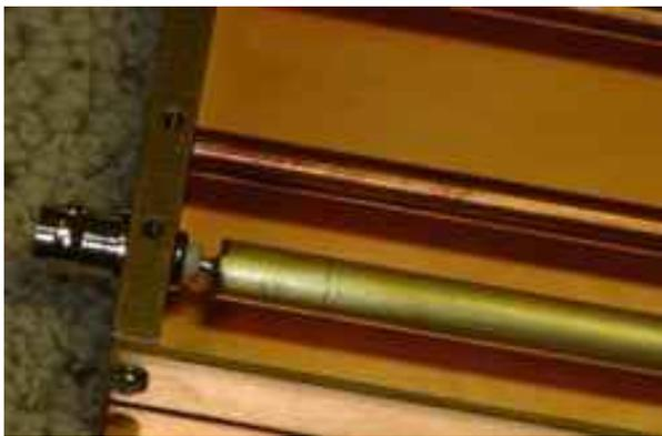
Fig. 4 BNC connector & input resonator
