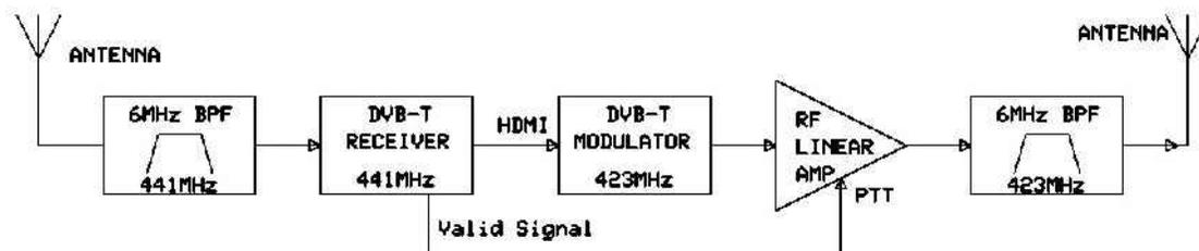
Fig. 1 A 70cm, Digital TV Repeater, block diagram.
