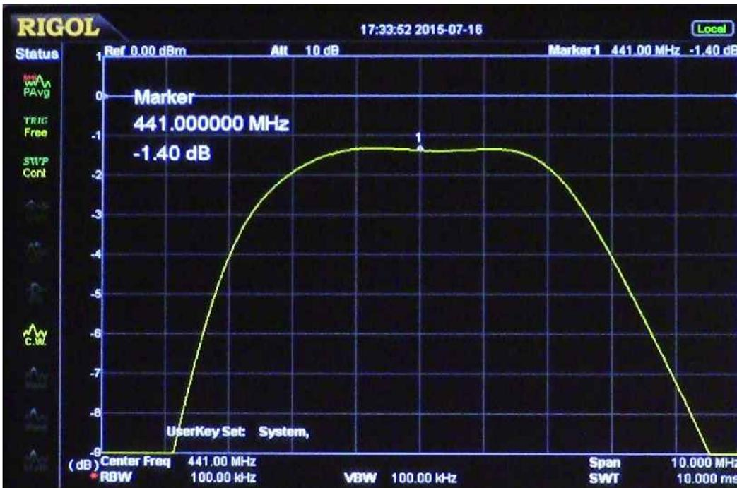
Fig. 10 Frequency Response of actual filter built by N0YE per Fig. 9 dimensions.
