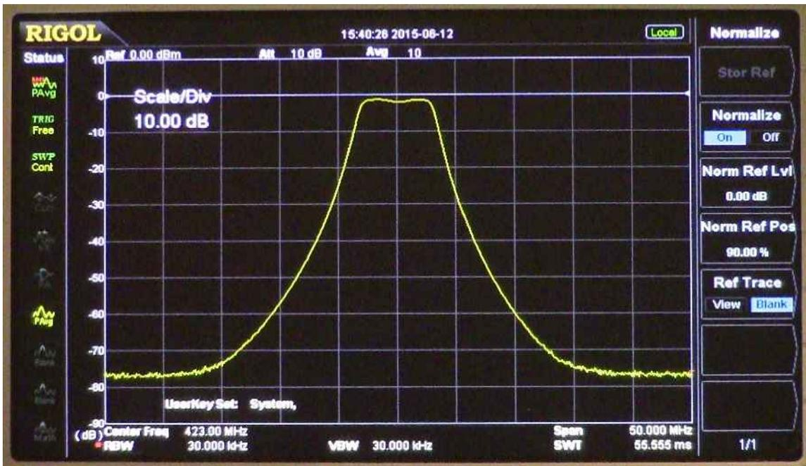
Fig. 7 Channel 60 SI-BPF --- Out of Band Performance
