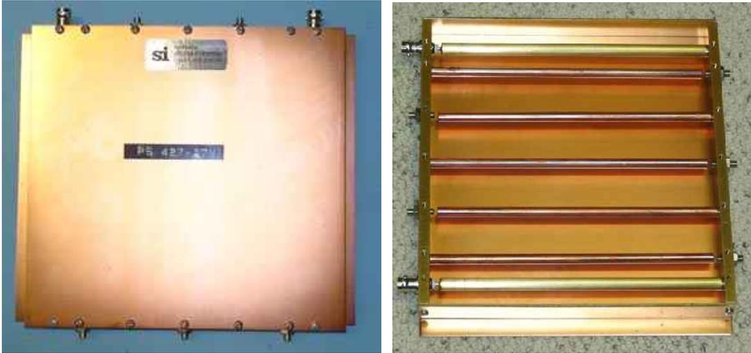
Fig. 3 Spectrum International, 70cm, ATV, Inter-Digital Band-Pass Filter
