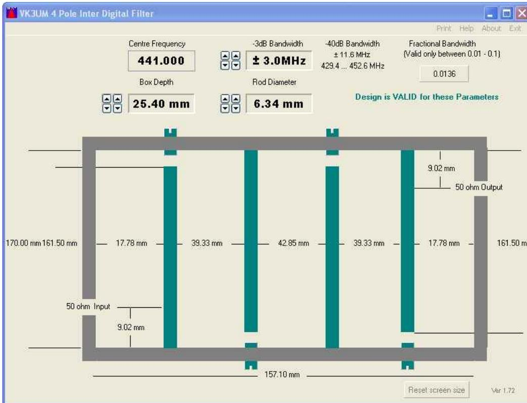
Fig. 9 VK3UM design for a 4 pole, channel 60 (441MHz), 6 MHz, Band-Pass Filter
