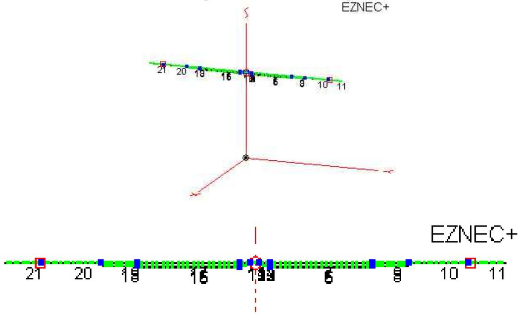
Fig. 3 Complete wire model of multi-band, dipole antenna.
