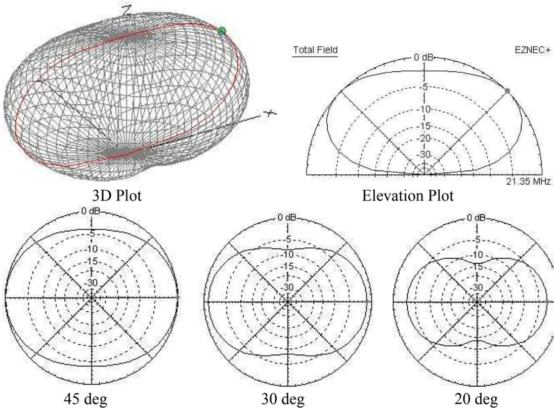
Fig.11 **15 meter**, 3D & 2D radiation patterns for multi-wire, horizontal dipole at 5 meters. vswr = 1.0461 Max. Gain = 8.2dBi at 45 deg. Gain = 6.0dBi (90deg), 7.4dBi (30deg) & 5.2dBi (20deg)
