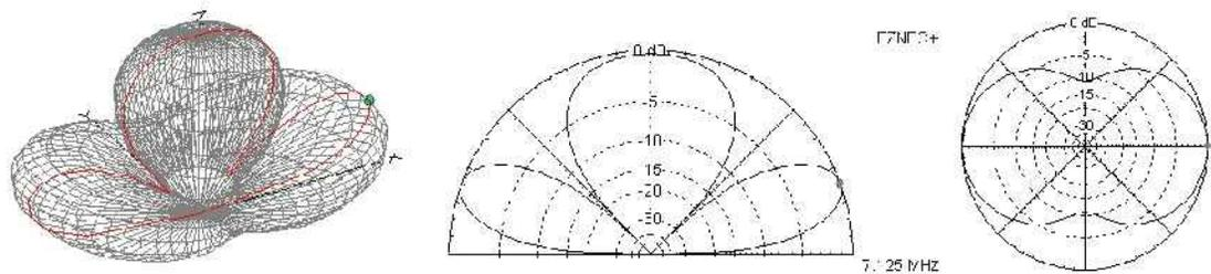
Fig. 8 **40m dipole antenna at 30 meter height.** 3D, elevation plot and azimuth plot (left to right). Max gain = 7.8dBi at 20 deg. Azimuth plot at 20 deg elevation.
