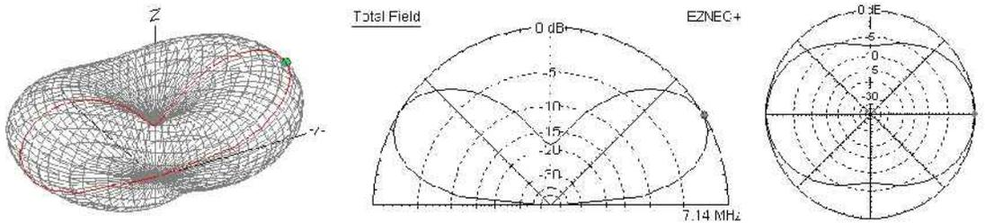
Fig. 7 **40m dipole antenna at 20 meter height.** 3D, elevation plot and azimuth plot (left to right). Max gain = 7.4dBi at 30 deg. Azimuth plot at 30 deg elevation.
