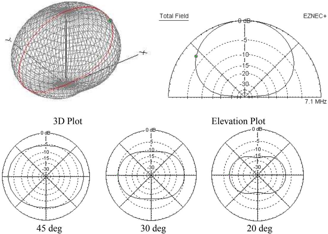
Fig. 9      **40 meter**, 3D & 2D radiation patterns for multi-wire, horizontal dipole at 5 meters. vswr = 3.6:1 Max. Gain = 9.2dBi at 90 deg. Gain = 6.7dBi (45 deg), 4.0dBi (30deg) & 0.9dBi (20deg)
