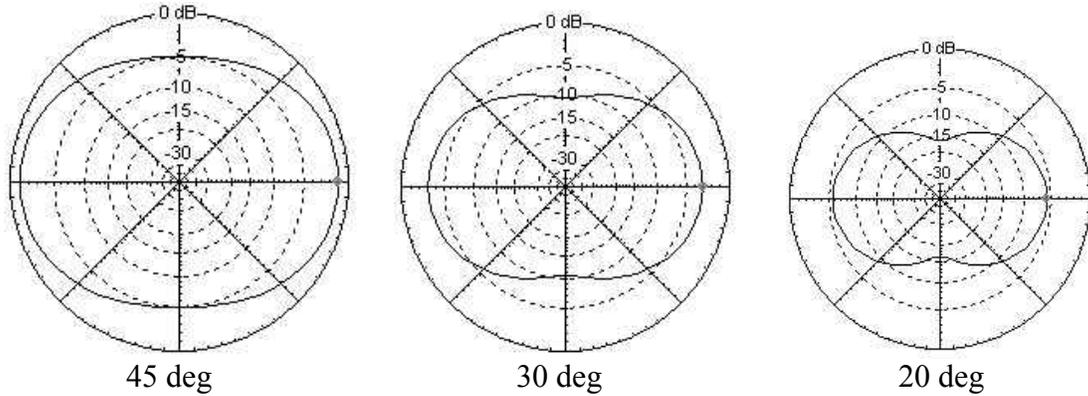
Fig.10 **20 meter**, 3D & 2D radiation patterns for multi-wire, horizontal dipole at 5 meters. vswr = 1.05:1 Max. Gain = 8.7dBi at 90 deg. Gain = 7.8dBi (45 deg), 5.7dBi (30deg) & 3.0dBi (20deg)
