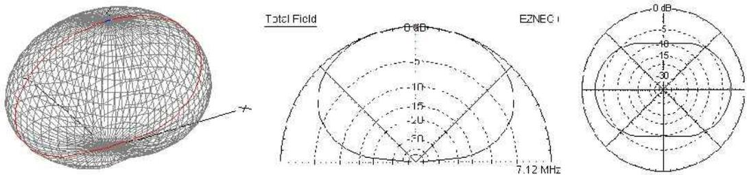
Fig. 6 **40m dipole antenna at 10 meter height.** 3D, elevation plot and azimuth plot (left to right). Max gain = 7.0dBi at 90 deg. Azimuth plot at 30 deg elevation.
