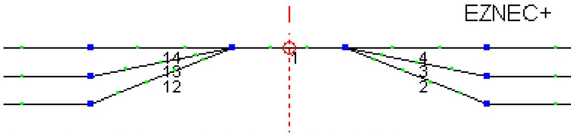
Fig. 2 Wire model for center feed-point of multi-band, dipole antenna.
