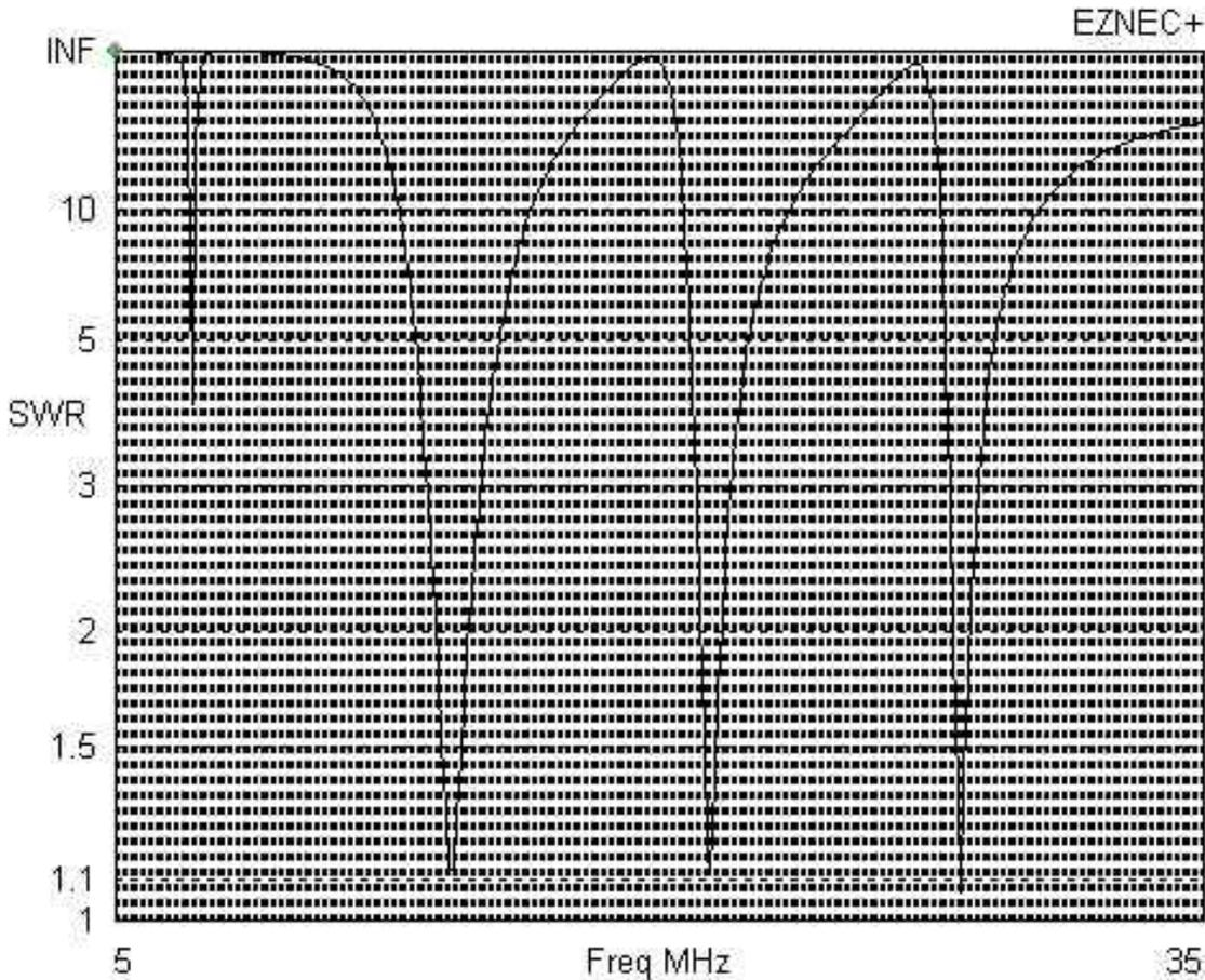
Fig. 4 Swept frequency calculation of antenna's VSWR.
