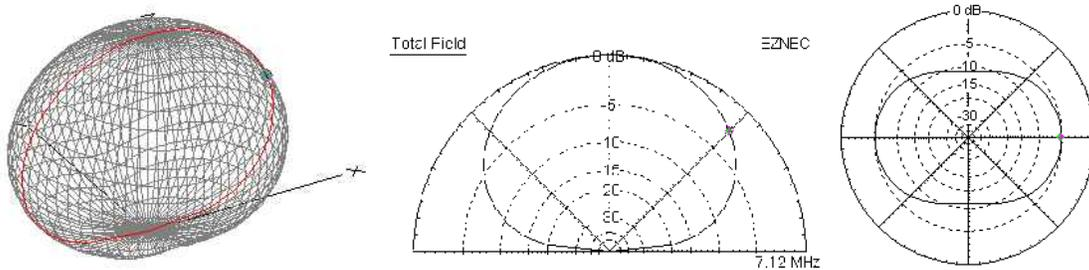
Fig. 5 **40m dipole antenna at 5 meter height.** 3D, elevation plot and azimuth plot (left to right). Max gain = 7.8dBi at 90 deg. Azimuth plot at 30 deg elevation.
