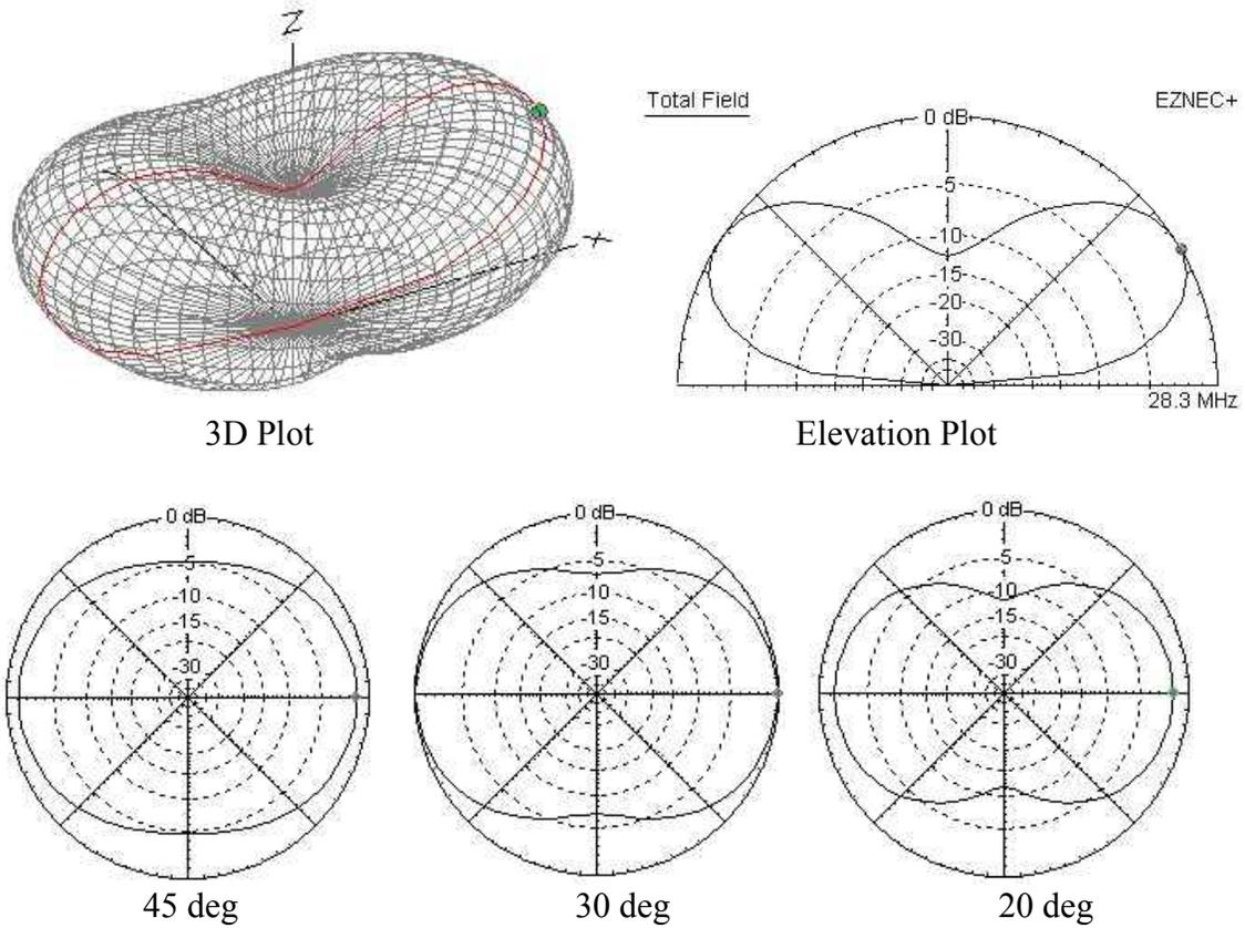
Fig.12 **10 meter**, 3D & 2D radiation patterns for multi-wire, horizontal dipole at 5 meters. vswr = 1.12:1 Max. Gain = 8.1dBi at 30 deg. Gain = -4.2dBi (90deg), 7.0dBi (45deg) & 6.7dBi (20deg)
