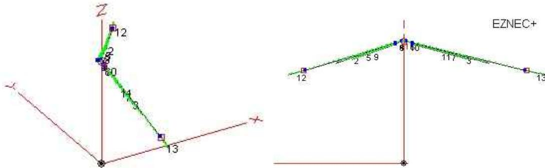
Fig. 16 Two views of the EZNEC wire model for the skewed, inverted V antenna.
